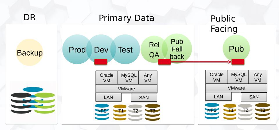
T1 SSD/Flash T2 Hybrid Flash/Conventional Disks T3 Conventional Disks
